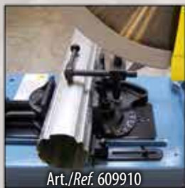
Art./Ref. 609910 ezentrishes Spannsystem eccentric clamping system
