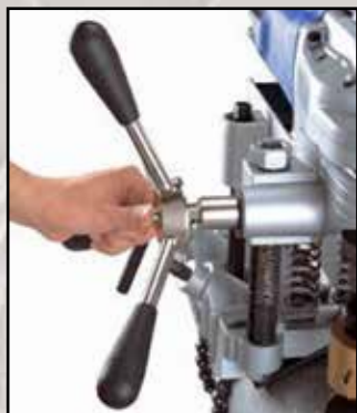
The tool free quick-release handle can be mounted on either side
